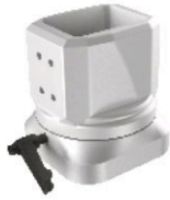
Item No./Name: Cabinet Connector Material: Die-cast Aluminum Alloy Rotation Angle: 0-320° Rotation Adjustment: With Locking Handle
